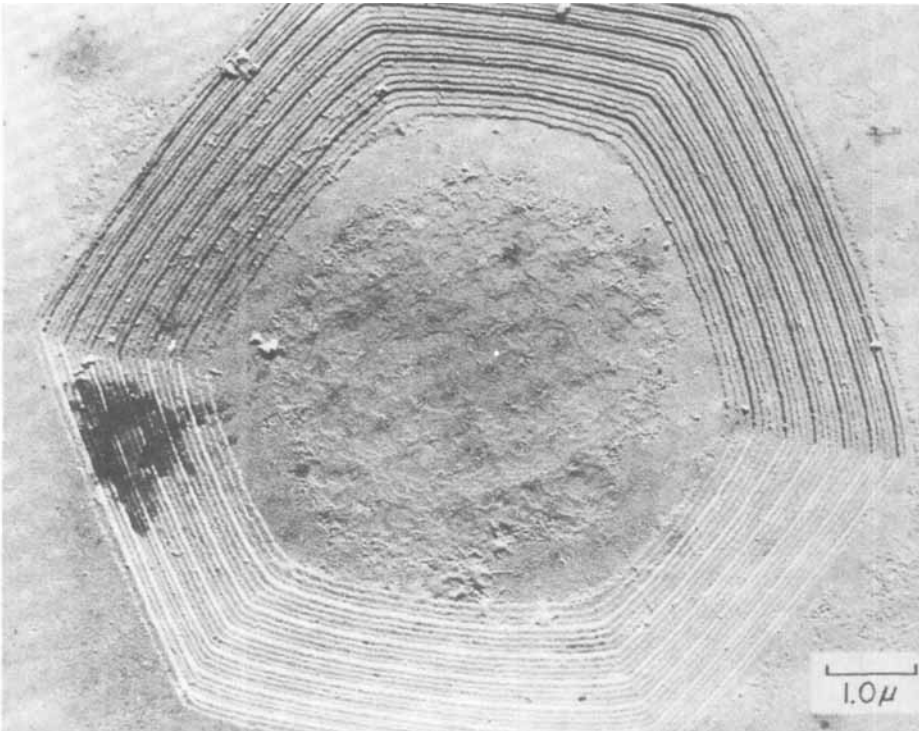
Figure 13. An etch pit on a crystal of a barium ferrite showing that the crystal contains a long repeating sequence of layers. This was shown to be MYYYYYYYYMYMYMYYYY (see figure 12), the depths of the steps corresponding to the blocks of Y-units (Kohn et al. 1967).
